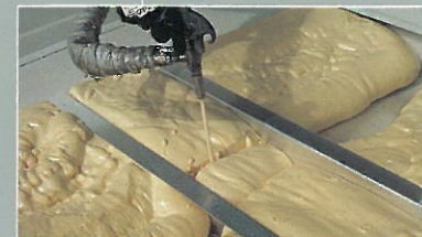
All Crestliners meet or exceed Coast Guard flotation regulations and we do it with form-fitting foam to deaden sound and add rigidity.
