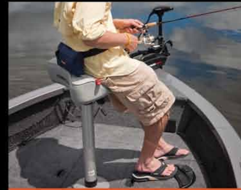
BUTT SEAT Crestliner's Butt Seat gives fishermen a sturdy spot to sit or lean against (when rotated 180 degrees).
