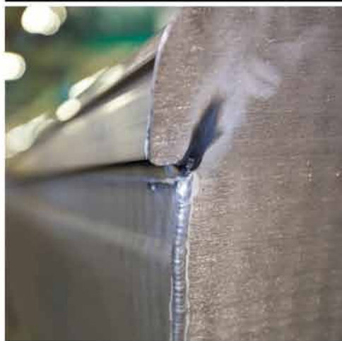
TOP LEFT: Once a hull is assembled, it gets sanded, prepped and sent to the paint room. RIGHT: Four large pieces of aluminum, joined together by continuous-seam welds, make up Crestliner's Four-X-Hull design.
