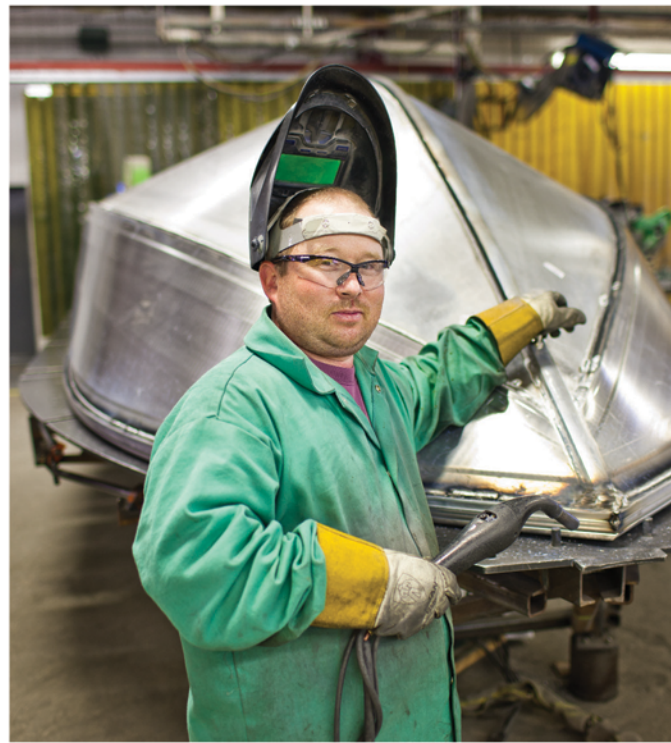
ABOVE: A member of the welding team at Crestliner's manufacturing plant in Minnesota stands with a freshly assembled hull. RIGHT: A welder at work on a stringer system. Aluminum arrives to the plant in massive rolls, which Crestliner then custom cuts and shapes in-house.
