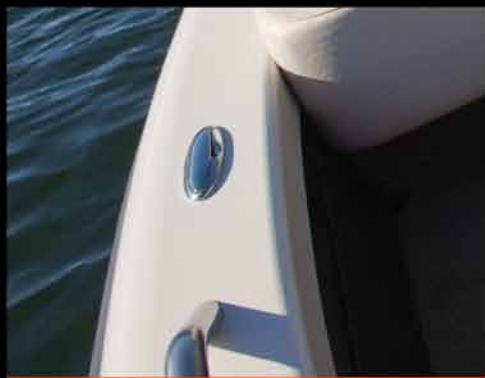
RETRACTABLE CLEATS Stainless steel Retractable Cleats recess flush into the gunnel when not in use.
