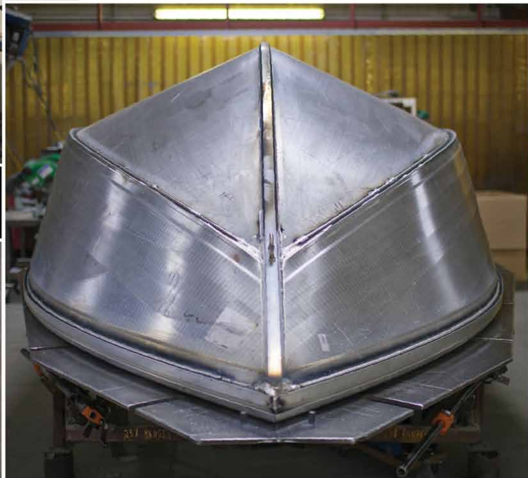
TOP LEFT: Once a hull is assembled, it gets sanded, prepped and sent to the paint room. RIGHT: Four large pieces of aluminum, joined together by continuous-seam welds, make up Crestliner's Four-X-Hull design.
