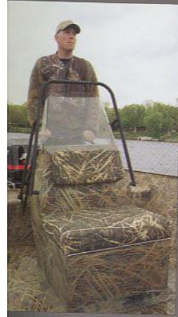
The Deluxe center console (VDC) has a grab rail and padded passenger seating
