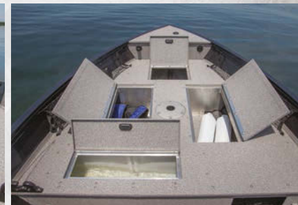
Large bow has 11-gal. aerated livewell, two large storage compartments, battery storage and cubby.
