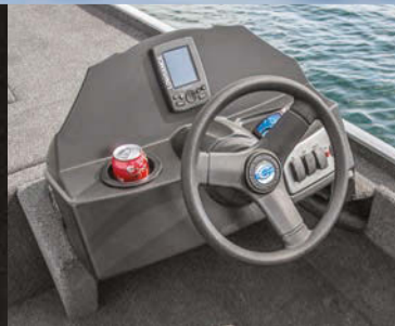
Console includes switch panel, cup holder and in-dash fishfinder.
