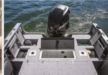
Stern casting deck with four compartments, livewell and OB-only optional conversion bench.
