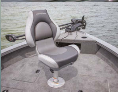
Spacious bow casting platform with pedestal base, storage and 12-gal. livewell.
