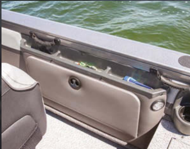
Under-gunnal starboard storage with door and topside quick-access trays.
