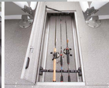
Locking in-floor storage compartment includes a rod rack accommodating five 7' rods.
