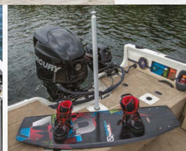
Stern platform may be outfitted with removable ski pylon (standard SST, optional OB).
