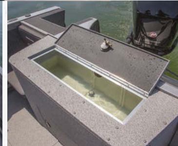
An aerated 20-gal. stern livewell comes with a timer to keep fish fresh.
