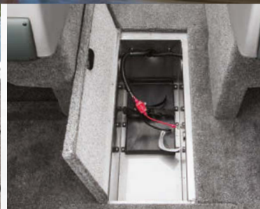
In-floor trolling motor battery storage compartment (24V system compatible).
