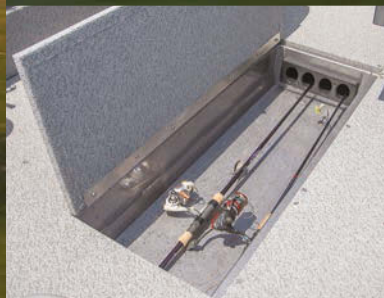
Center in-floor locking rod storage with four tubes. (1650: 9' capacity; 1450: 7' capacity)
