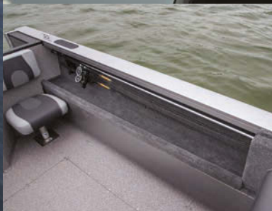
Starboard/port rod storage with four 9'6" rod tubes and open storage below.
