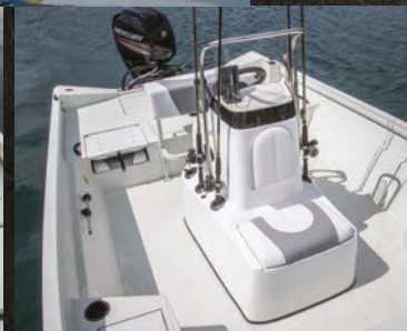
Fiberglass center console with leaning post, vertical rod holders, windscreen and forward seat. (2000)
