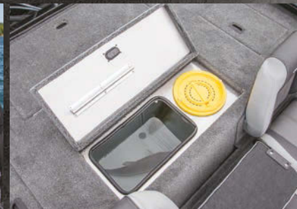
The aerated 22-gal. stern livewell includes a timer and space for a bait bucket.
