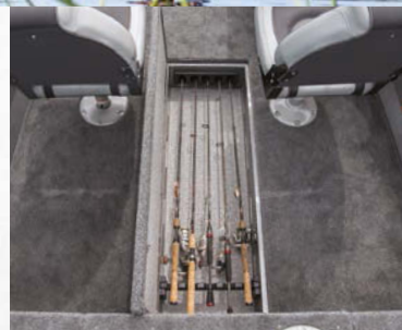
Spacious lockable in-floor rod storage holds five 9' rods. (1600)
