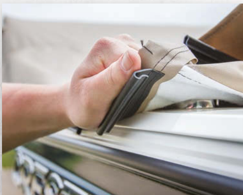
TRAVEL COVER WITH J-HOOK The snug, custom-cut travel cover attaches securely to extruded gunnels with easy on/off snapless J-Hooks. Walk-through models have a new ratchet design without poles.
