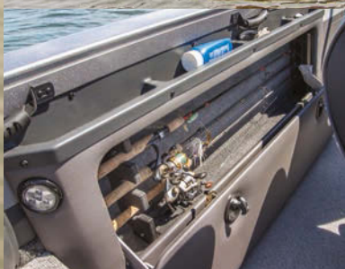
Vinyl-wrapped port rod box with topside trays (OB: four 8' capacity; SST: four 7'6" capacity).
