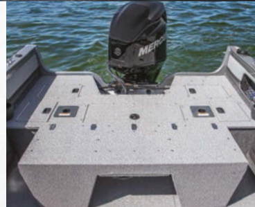
Stern casting deck with two pedestal seat bases extends with OB-only optional conversion bench.
