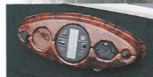
Built-in bow electronics panel is standard. Optional electronics package features Zercor locator (shown) and Motor Guide trolling motor.
