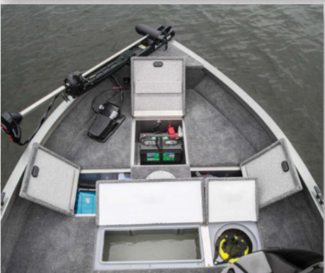
Bow casting platform loaded w/ in-floor storage includes a 19-gal. aerated livewell.
