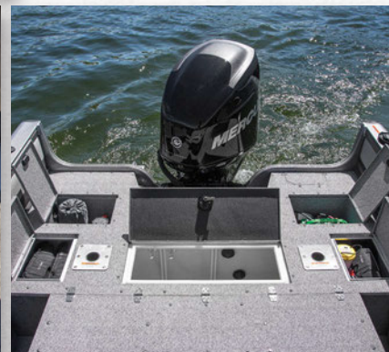
Stern casting deck w/ four compartments, live-well and OB-only optional conversion bench.
