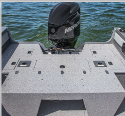
Stern casting deck w/ two pedestal seats extends w/ OB-only optional conversion bench.
