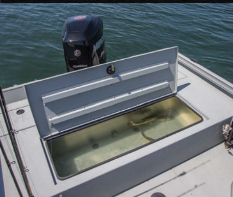
The 100-gal., 64" dual-pump stern livewell accommodates trophy catches.
