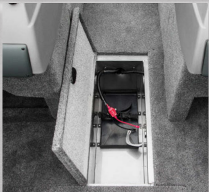
In-floor trolling motor battery storage compartment (24V system compatible).
